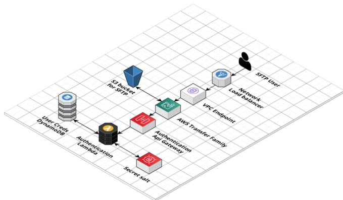
As you can see from the schema, we had to introduce a couple of unexpected services such as a Network Load Balancer, and a VPC endpoint. These two components are needed to make sure that the exposed IPs are fixed and will never change. In fact, in this way it's possible to allocate an Elastic IP, also enabling you to use an IP address that you own (BYOIP). This feature is commonly required for specific problems with firewall rules.
