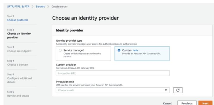
API Gateway (configuration steps can be found [here](#)) must expose an API backed by an AWS Lambda. This API will be called by AWS Transfer Family to check the credentials of the user that made an FTP request to the service.
